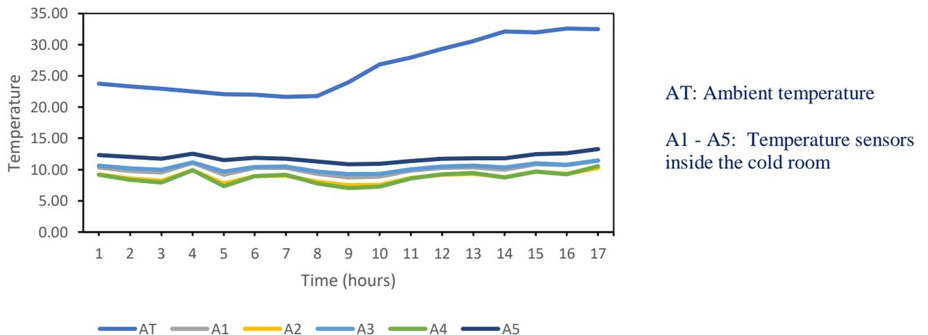
Figure 7-1: Temperature variations with out fresh produce.
