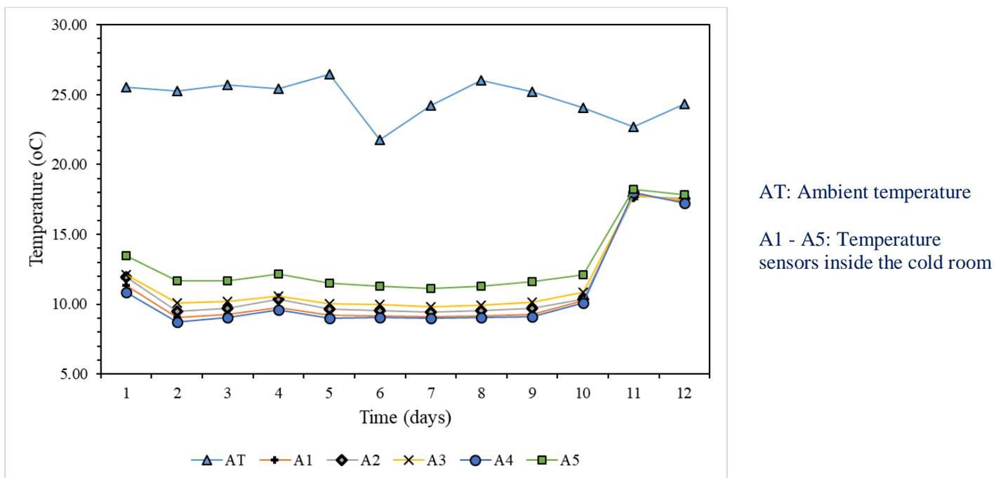
Figure 7-2: Temperature inside the cold storage as a function of time
