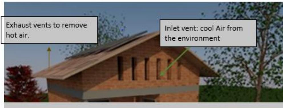
Figure 6-2: Attic with air vents.
