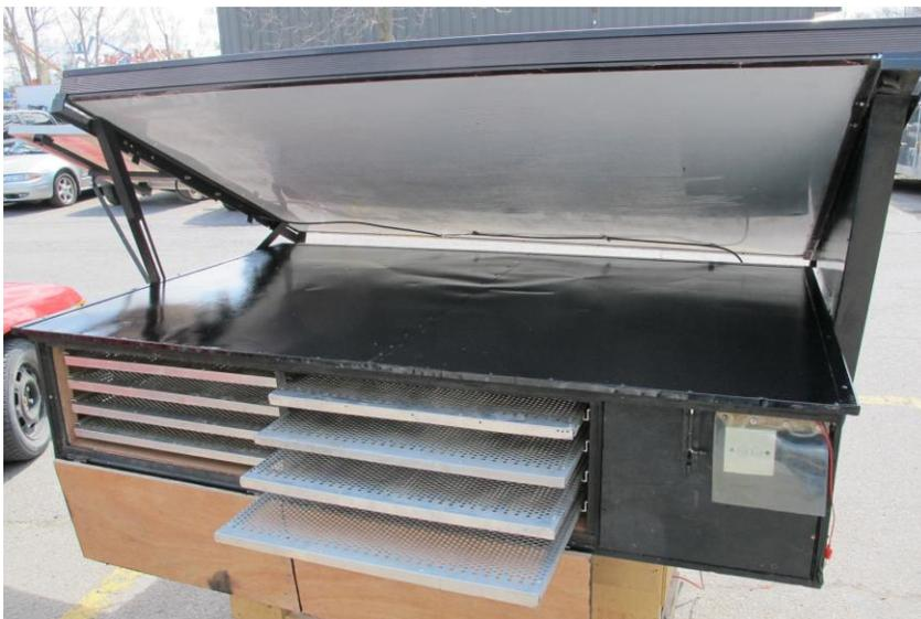
Rear view showing cabinet doors, aluminum racks and fan switches.
