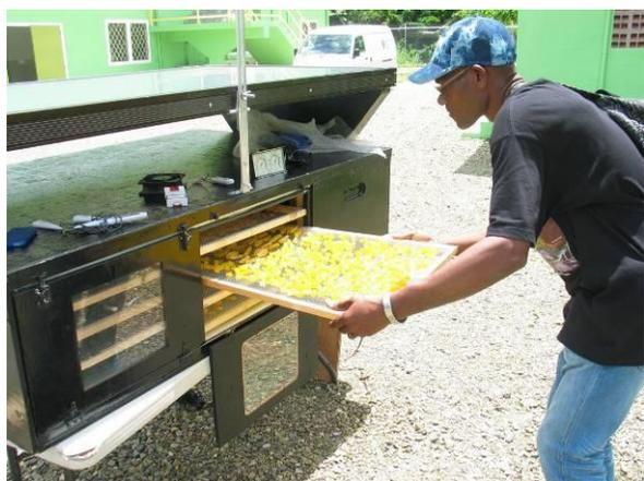
Temperature ranges of 40 – 70 C will effectively kill bacteria and inactivate enzymes, although temperatures of approximately 45 degrees are recommended for solar dryers. This temperature is easily achievable in the SolarFlex dryer as it will normally deliver temperatures of about 25-30 degrees higher than the outside temperature.
